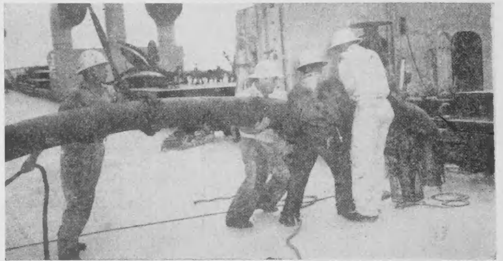
The midpoint of turnaround comes when the wharfingers fasten the hose to the deck connections of a tanker. Coordination of all factors makes fast turnaround possible.
